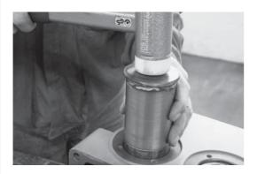
Put the assembly sleeve on the bearing outer ring and drive the bearing outer ring into the housing.
