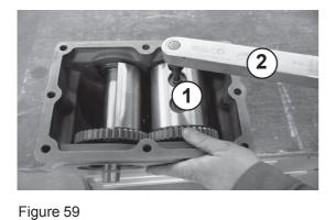
Fit the eccentric (59/1) by means of a dynamometric key (59/2).
