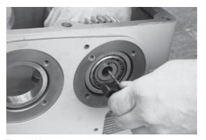
Loosen the fastening pin of the control pin.
