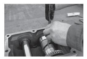
The cut surface of the control pin must point towards the adjusting pin.
