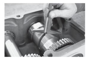
Ensure that the control pin runs approximately 1,5mm beneath the upper edge of the groove of the adjusting gear wheel.
